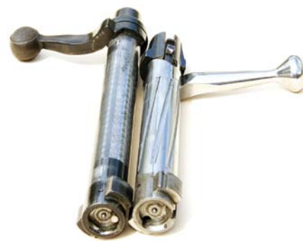
A Remington and a PTG bolt fresh from the hunt, with plenty of accumulated crud showing. Oil-based bolt lubes will exacerbate this situation by attracting dust and grime.
